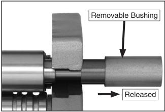
Figure 30. Removable bushing release.
